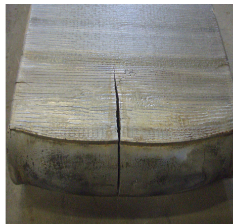
Energy expended to remove cracks in aluminum ingots to meet high quality standards costs the U.S. aluminum industry millions of dollars annually.
