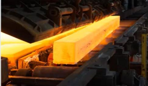
Semi-finished steel is reheated using a dynamically controlled process before entering the hot rolling operations. Reheating uses 70-80% of total energy used in rolling mills.
