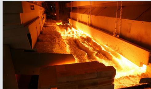
Raw materials entering a float-glass furnace tank for production of architectural glass. *Photo from Vitro Glass.*
