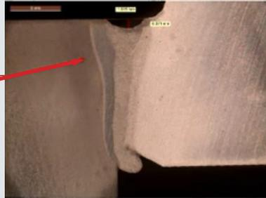
Full penetrating lap welds for transmission sun gear assembly
