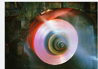
Hot rolling process is used to produce sheet steel. Photo from AK Steel.
