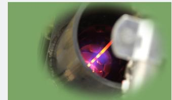
Experimental combustion rig is used to determine emissions under various conditions. Photo from VAST Power Systems.
