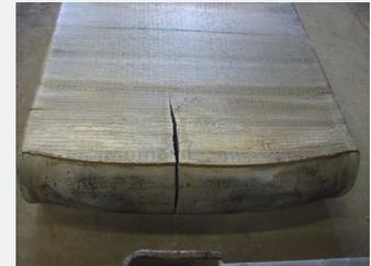
Cast aluminum ingots will crack if the process conditions are not optimal. Photo from Arconic Aluminum.
